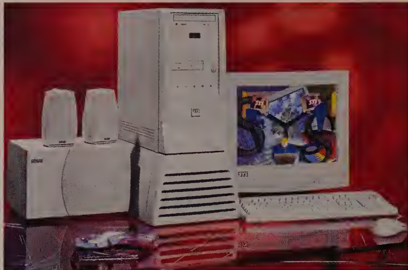
CHILL OUT: A base unit cools the overclocked CPU of Sys's Cold Fusion, which set a PC WorldBench 98 record for a PC running Windows 98.
